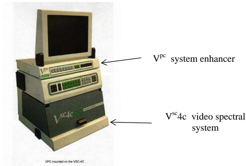
This unit enables the user to conduct incident and transmitted visible and/or infrared, short and/or long wave ultraviolet light, oblique light, and coaxial lighting for retro-reflective security feature examinations on documents. The resulting images can be imported to a computer for future use.. Most of the images in this paper are from this instrument.
